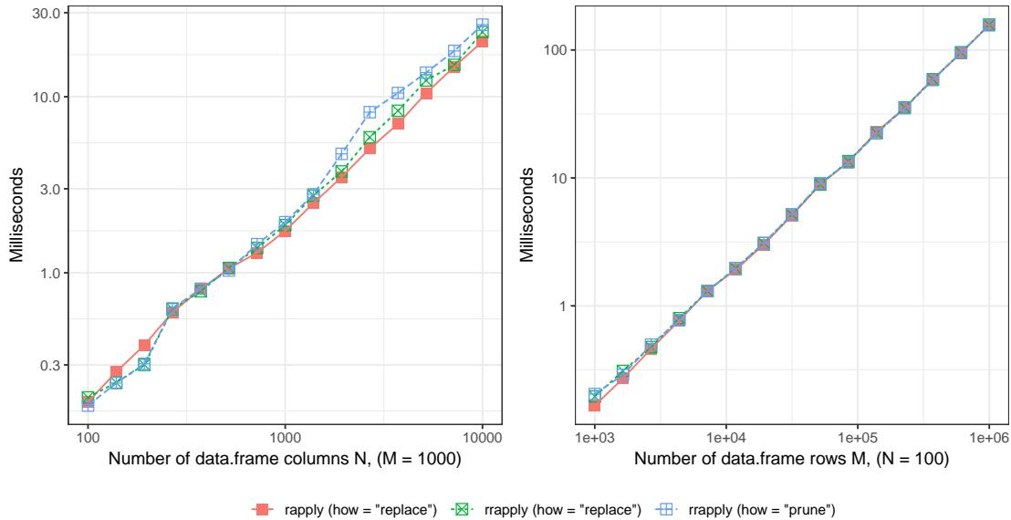
Benchmark timings: mutating all numeric columns ( $M \times N$ ) –sized data.frame
